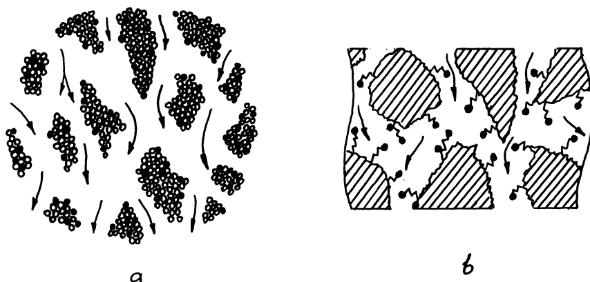
Figure 22. Structure of the perfusion sorbent (a) and PGMA-EDMA -G grafted membrane (b). Filled circles are functional groups (adsorption sites) .
